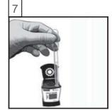
Empty the pipette into the sample chamber.
