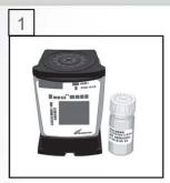
Obtain one Xpert cartridge and one Sample Reagent vial for each sample.
