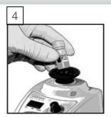
Recap the Sample Reagent vial and vortex for 10 seconds.
