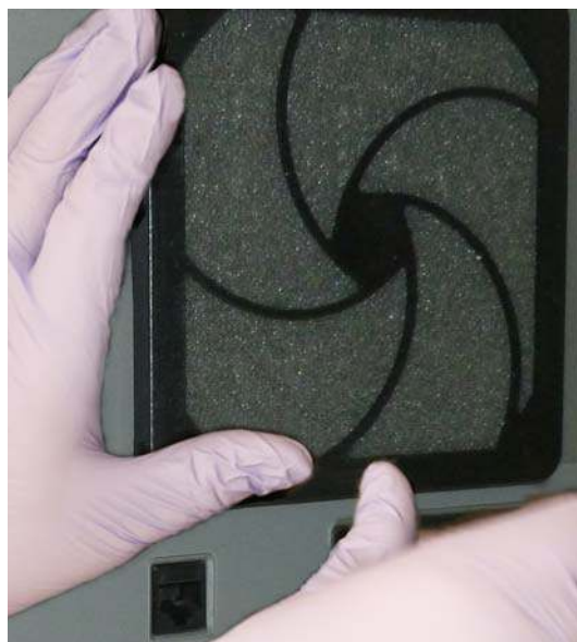
GeneXpert Xpress II: Pressing the Bottom into Place
