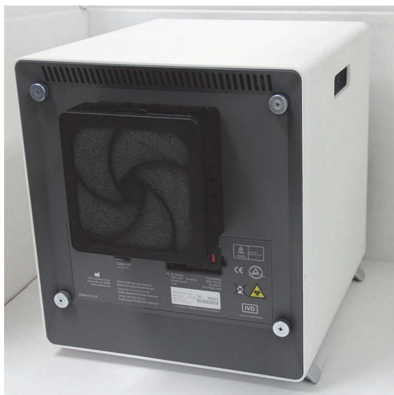
Figure 9-17. GX-IV Instrument Positioned for Access to Filter
