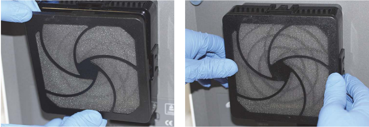
Figure 9-24. Replacing the Prefilter and the Prefilter Retainer
