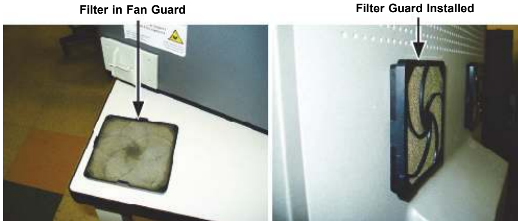
Figure 9-13. Replacement Filter and Guard Installed
