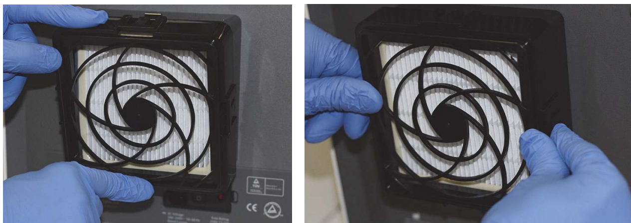
Figure 9-23. Replacing the HE Filter Retainer
