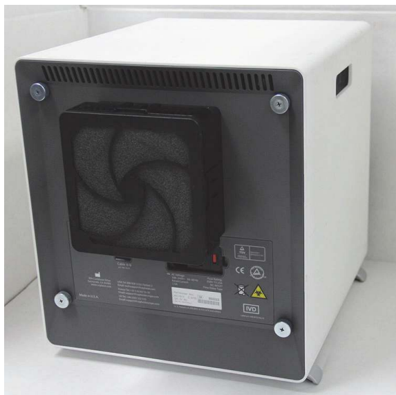
Figure 9-17. GX-IV Instrument Positioned for Access to Filter
