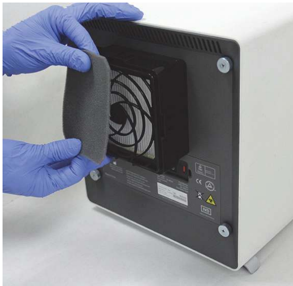
Figure 9-19. Removing the Prefilter
