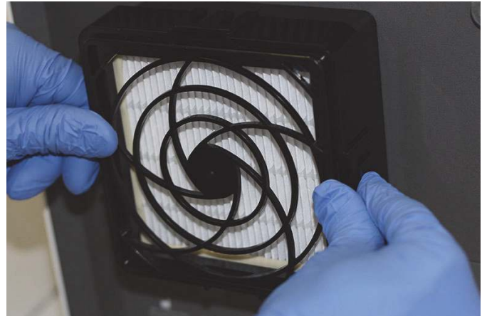
Figure 9-23. Replacing the HE Filter Retainer
