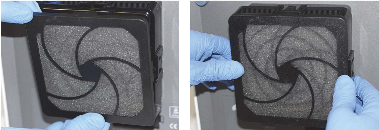
Figure 9-24. Replacing the Prefilter and the Prefilter Retainer
