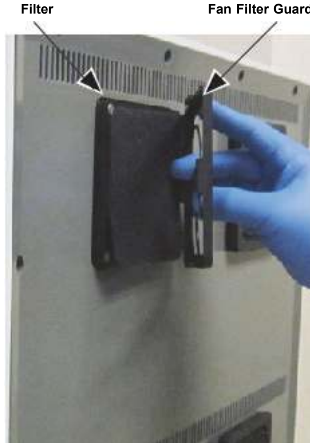
Figure 9-15. Removing the Fan Filter Guard and Filter
