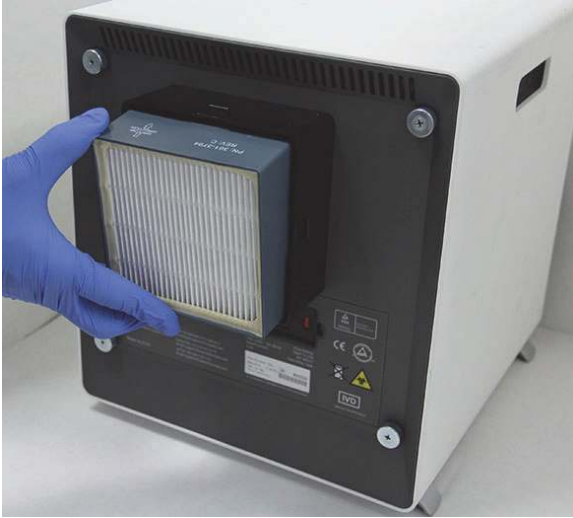
Figure 9-22. Replacing the HE Filter
