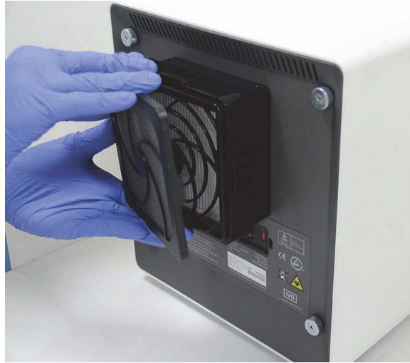
Figure 9-18. Removing the Prefilter Retainer
