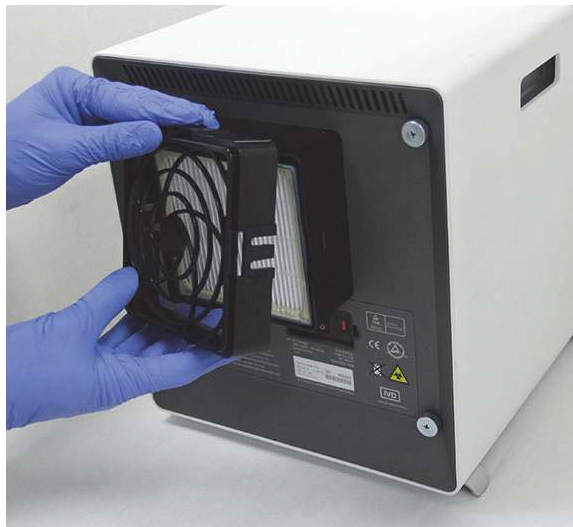
Figure 9-20. Removing the HE Filter Retainer
