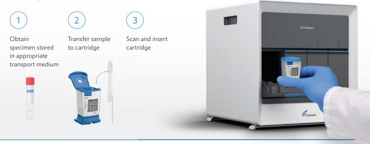
**Xpert**<sup>®</sup> **Xpress SARS-CoV-2/Flu/RSV** is a qualitative real-time PCR test that provides accurate detection and differentiation of SARS-CoV-2, Flu A, Flu B, and RSV in as little as 25 minutes.\*
