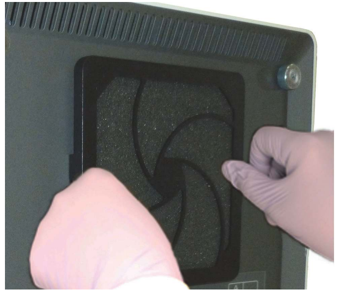
GX-IV: Pressing the Sides into Place
