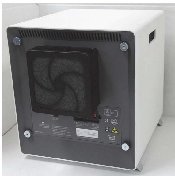
Figure 9-17. GX-IV Instrument Positioned for Access to Filter
